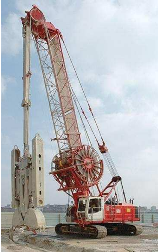
KS 3000 hydraulic grab for diaphragm walls and barrettes
